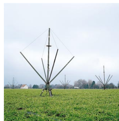
FIG 4 HF DF Antenna ADD011 (0.3 to 30 MHz, correlation method) Photo 42 342
