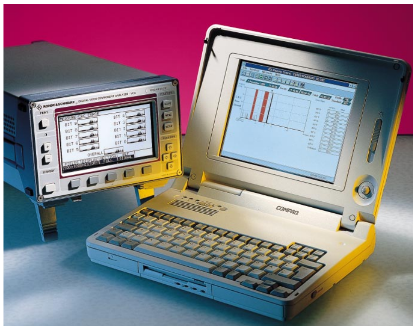
FIG 1 VCA and PC performing digital serial video-signal monitoring round the clock Photo 42 331
