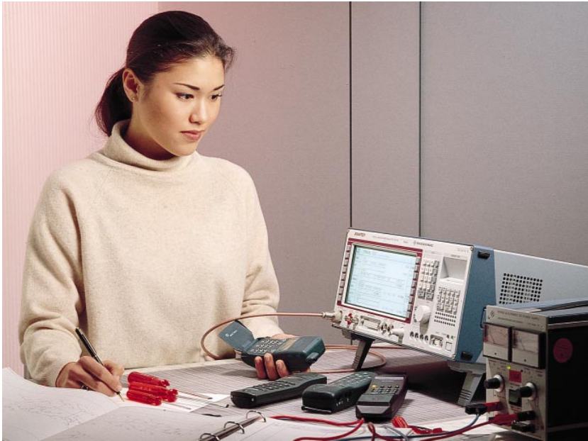
Digital Radiocommunication Tester R4860, compact tester based on CMD units, for transmitter and receiver tests on mobile phones of Japanese network PDC Photo 42 333/1
