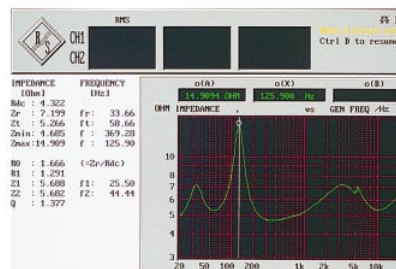
FIG 2 Impedance characteristic with test report (resonance frequency and impedance, resistance, Q, etc)
