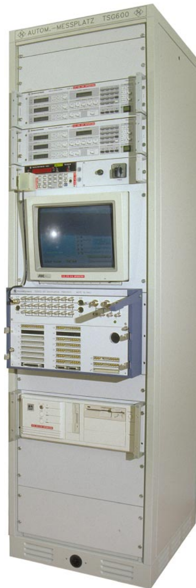
FIG 2 TSU system can be integrated in 19-inch rack for applications requiring lots of add-on units.
