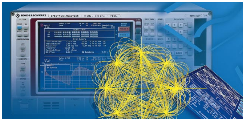
FIG 1 Spectrum Analyzer FSE with vector signal analyzer option for measuring digital modulation parameters
