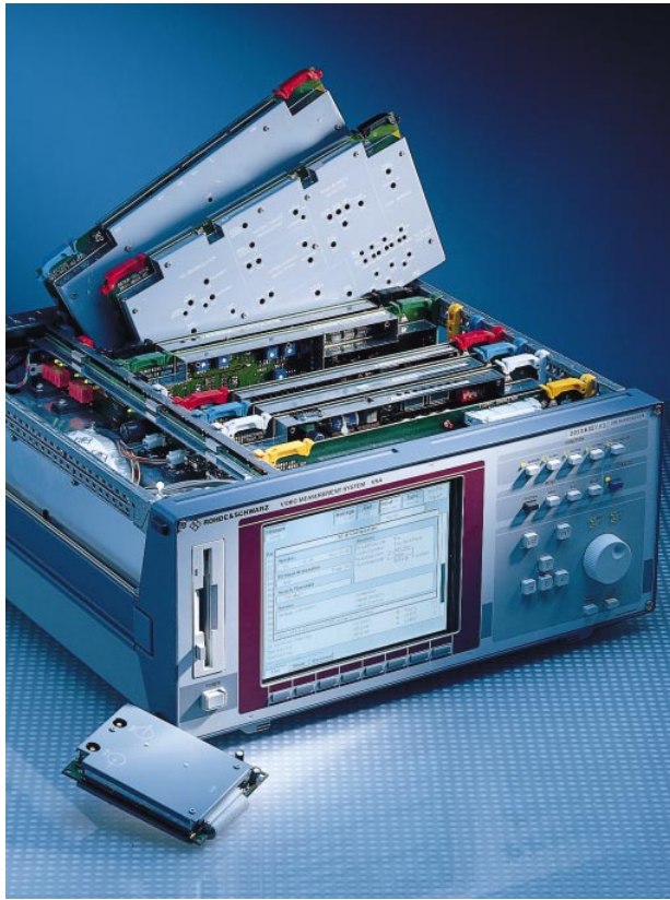
FIG 1 Video Measurement System VSA supports special test requirements of TV transmitters and cable systems with the aid of built-in test-receiver option (configuration menu of test receiver displayed) Photo 42 329/2
