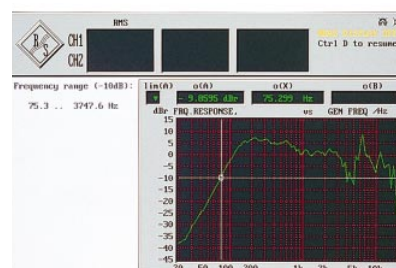
FIG 3 Frequency response and calculated frequency range of loudspeaker (to IEC 268, part 5)
